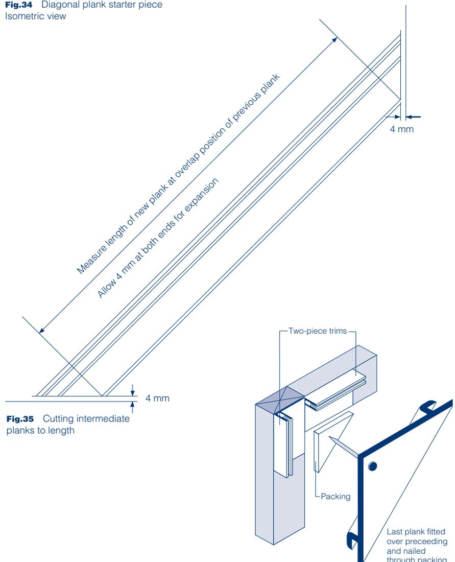
**Fig.35** Cutting intermediate planks to length
