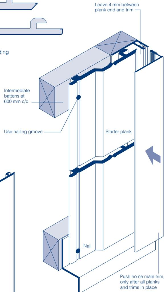
**Fig.32** Locating starter plank (working right to left)
