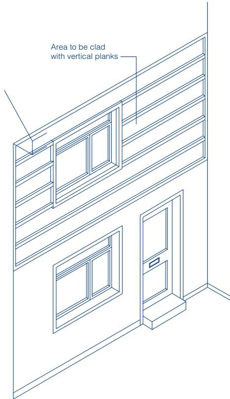
Fig. 23 Battening out
