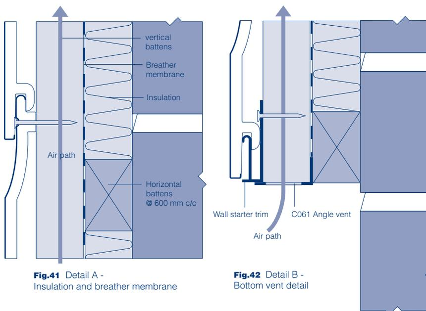
**Fig.41** Detail A - Insulation and breather membrane
