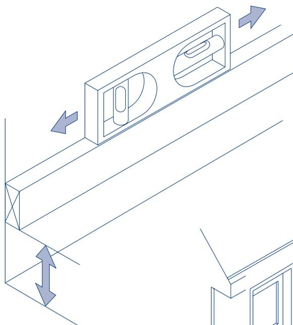
**Fig. 1** Check height, line and level of starter batten
