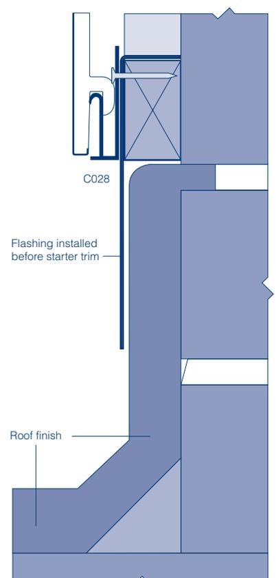
Fig. 7 Wall starter trim C028 above flat roof
