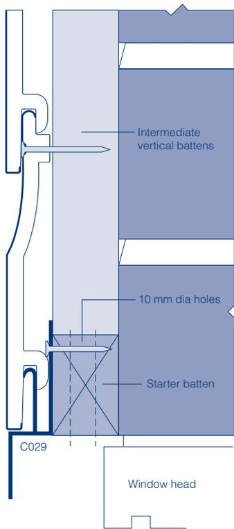
Fig. 6 Drip starter trim C029 at window head
