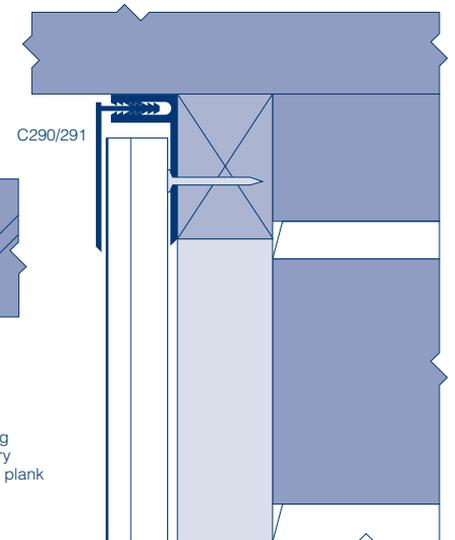
**Fig.28** Universal two-part trim C290/291 at head of cladding
