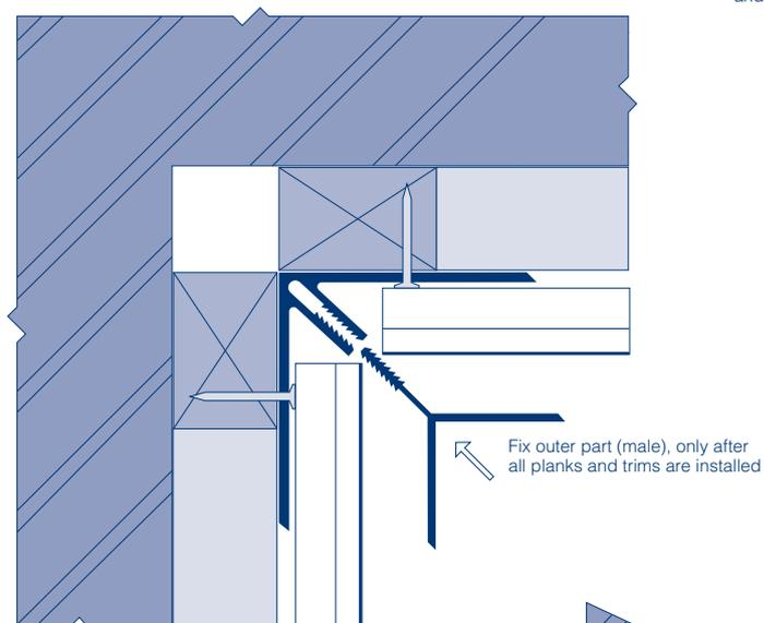
**Fig. 14** Two-part trim C292/293 at internal corner
