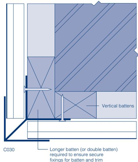
**Fig. 12** Corner trim C030 at an external angle
