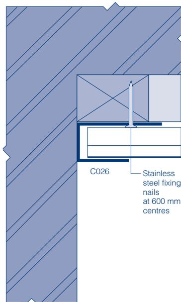
**Fig. 10** Universal channel C026 at cladding reveal
