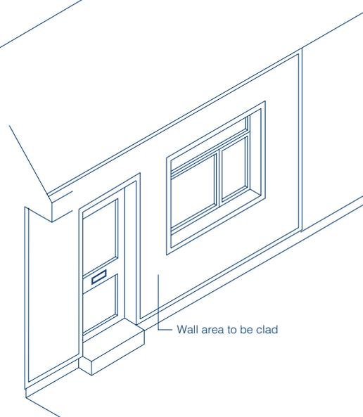
**Fig. 2** Batten out all perimeters and openings
