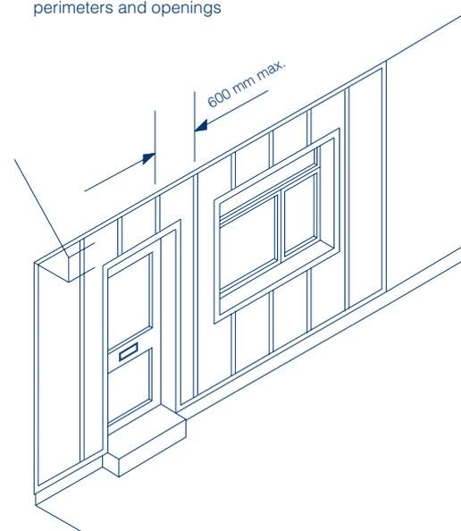
**Fig. 3** Fix intermediate vertical battens at 600 mm centres
