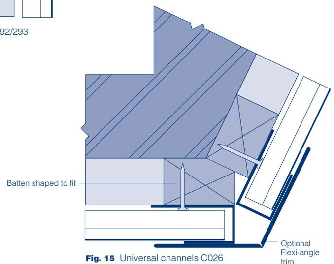
**Fig. 15** Universal channels C026 used back-to-back at external obtuse angled corner
